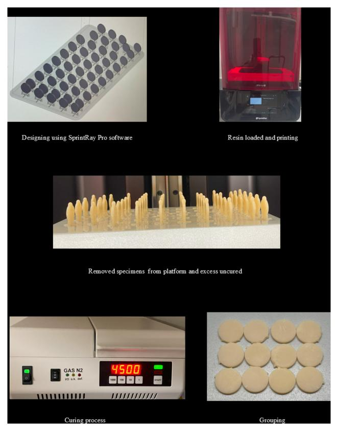
Fig. (3). Steps in specimen fabrication using sprintray printer.
