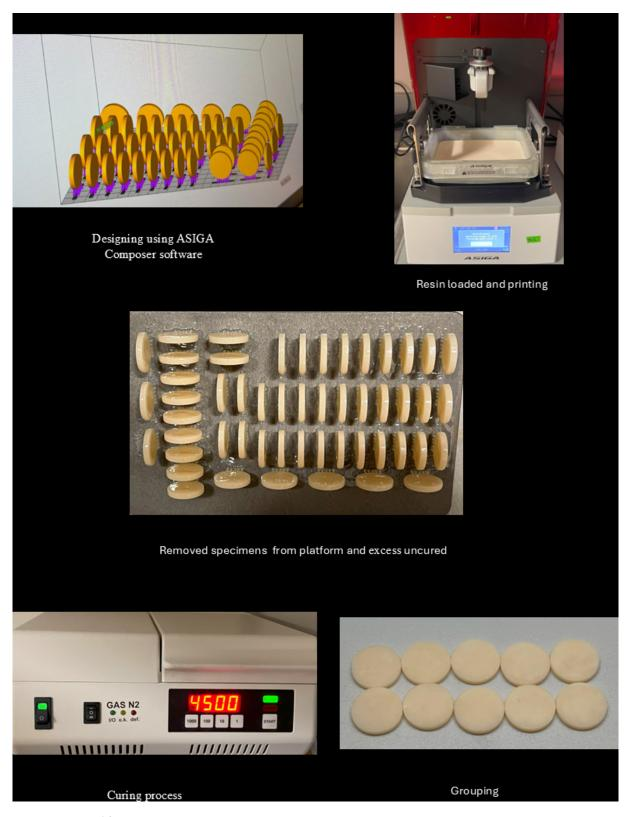
Fig. (2). Steps in specimen fabrication using asiga printer.
