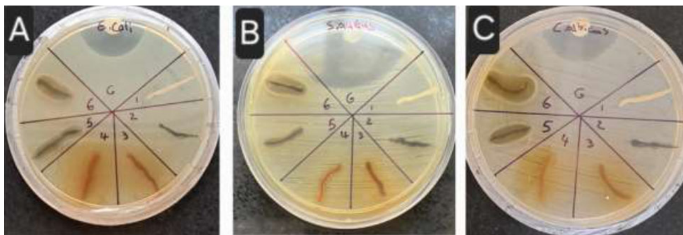
Fig. (7). 1: uncoated thread, 2: PDA coated thread, 3: coated with black tea extract, 4: coated with green tea extract, 5: Ce-BT+PDA coated thread, 6: Ce-GT+PDA coated thread. A: E. coli , B: S. aureus , C: C. albicans .
